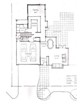
ABOVE FIG. 6-19: Compact medium density housing capable of being a fully self contained unit on the ground floor
